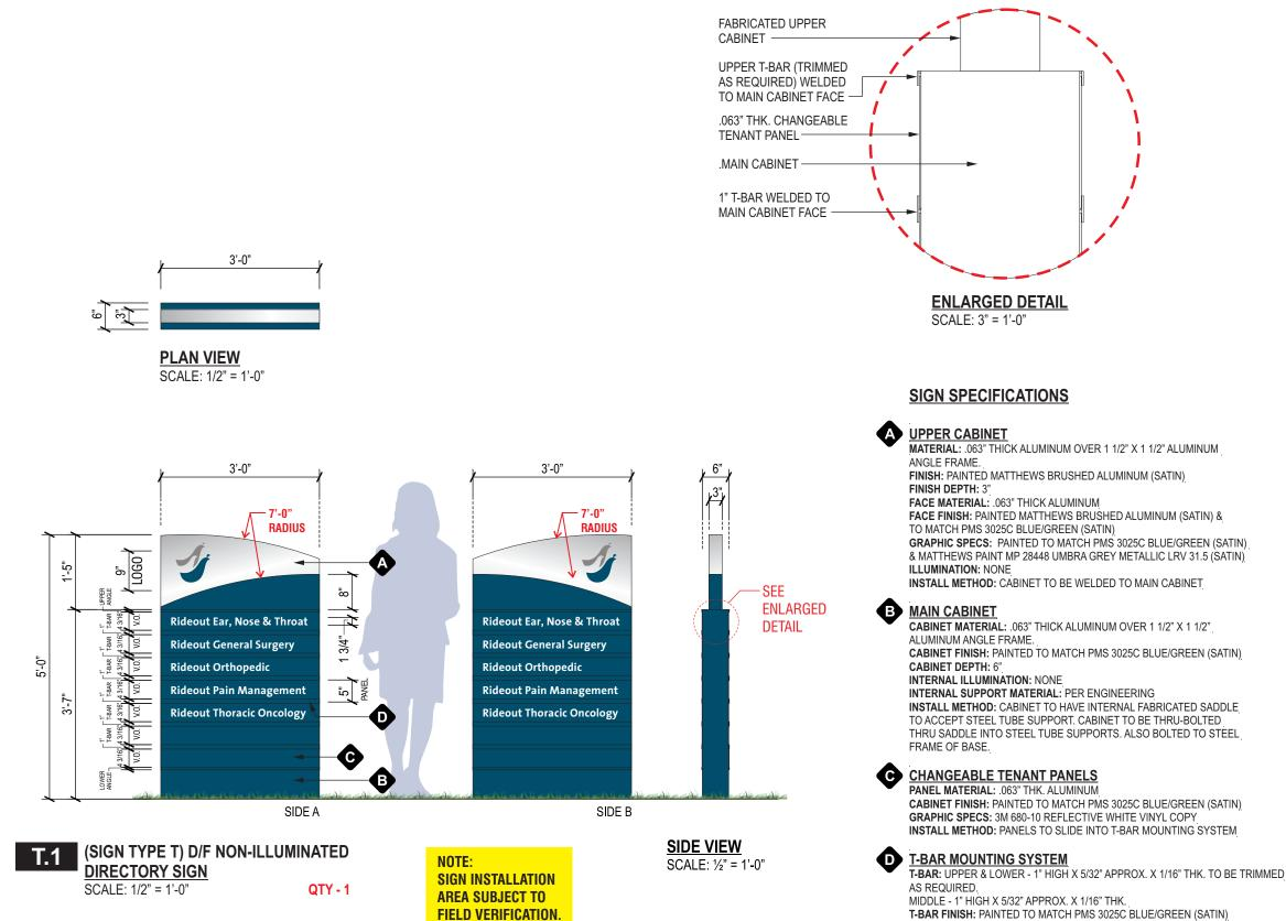
T-BAR FINISH: PAINTED TO MATCH PMS 3025C BLUE/GREEN (SATIN) INSTALL METHOD: TO BE WELDED TO MAIN PANEL
