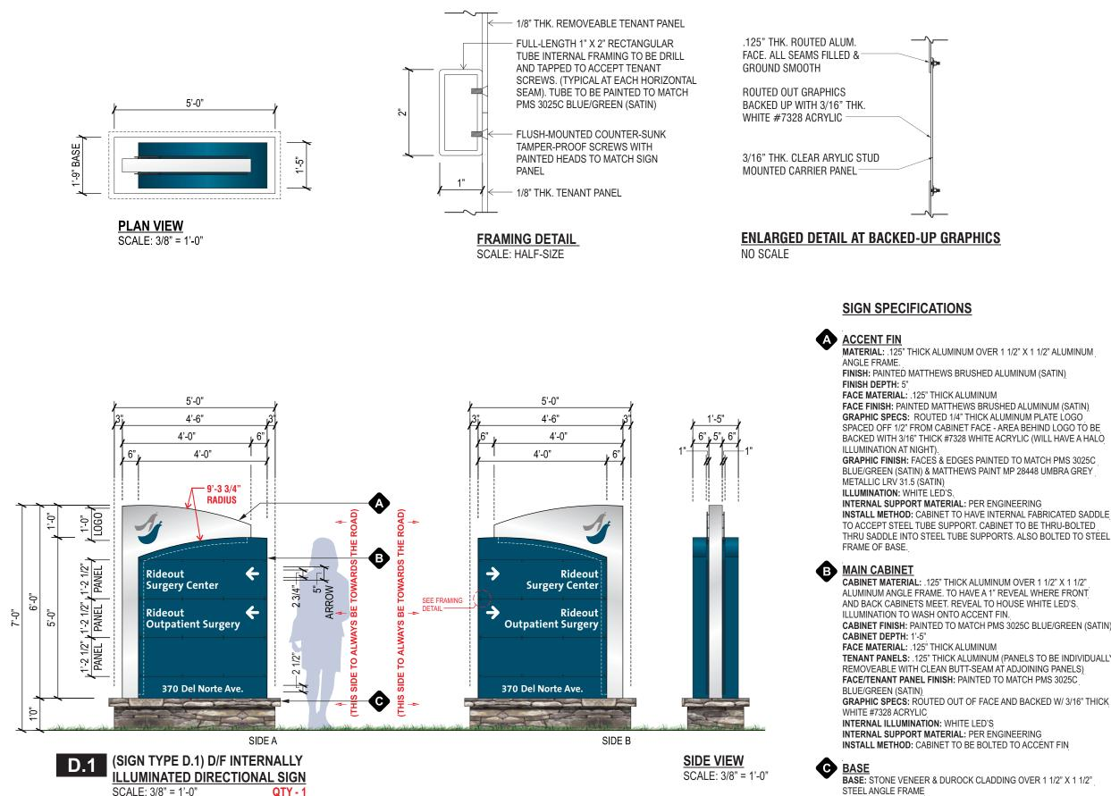
BASE: STONE VENEER & DUROCK CLADDING OVER 1 1/2" X 1 1/2" STEEL ANGLE FRAME VENEER SPECS: EL DORADO STONE - BLUFFSTONE MINERET TOP CAP: MT. MARRIAH MORTAR: BASALITE TYPE S 225 (GRAY)
